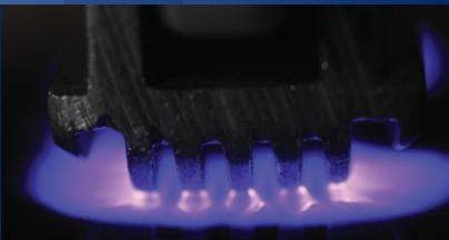
As one of the flagship technologies in our solution line-up, **CORONA** discharge treatment relies on a tried, tested and proven technique. Using the corona effect, an electrical phenomenon well known to physicists, we **considerably increase the wettability and adhesion coefficients** necessary for good surface bonding, **regardless of the composition and shape of your plastic substrates.**
